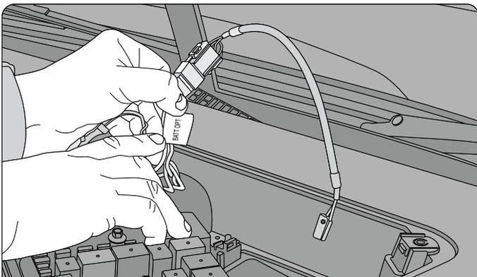
**Step 3:** Connect the 2-pin black power T-cable from the kit to the 2-pin power connector labeled BATT OPT.
