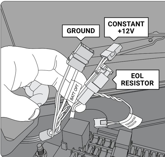
**Step 2:** Inside the fuse box, locate the connector labeled BATT OPT, and the terminating resistor. These will be used in later steps.
