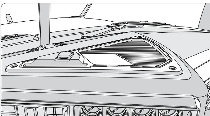
**Step 8:** Clean up all wiring using zip ties. Be sure not to obstruct any fuses. Complete an installation check for the GO device and then reinstall the fuse box cover.
