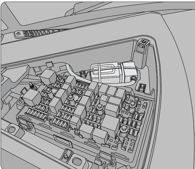
**Step 7:** Connect the HRN-CM24Y1 to the GO device. Secure the GO device to the harness using a zip tie. Secure the GO device to the frame of the fuse box using an additional two zip ties.
