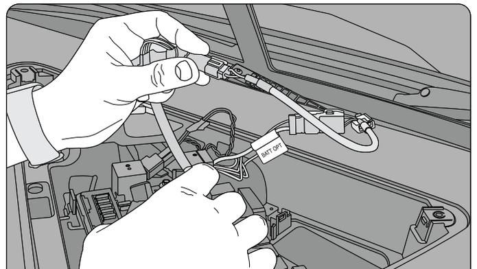
**Step 4:** Connect the other end of the T-harness to the HRN-CE10A2 harness.
