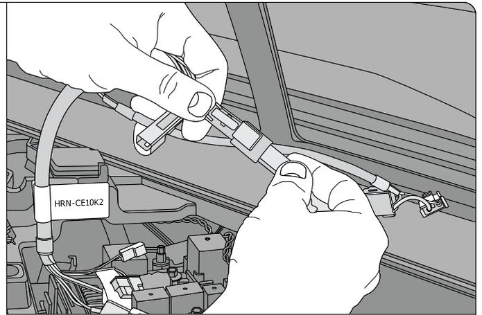
**Step 5:** Remove the terminating resistor and then plug it into the mating end of the HRN-CE10A2. Connect the HRN-CE10A2 to where the terminating resistor was removed.
