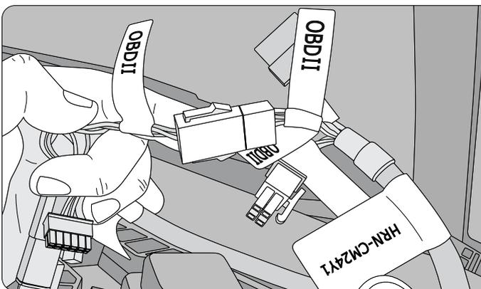
**Step 6:** Connect the 6-pin white Molex connector on the HRN-CE10A2 to the 6-pin white Molex connector on the HRN-CM24Y1. They are both labeled OBDII.
